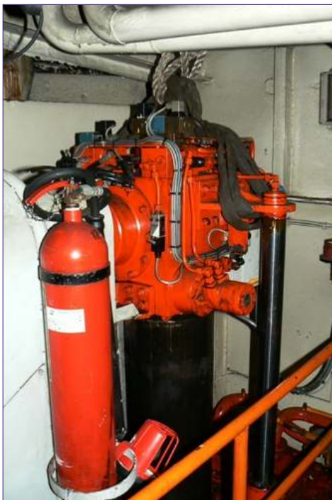
Veth 250hp hydraulic azimuth propellor, coupled to a V8 Iveco industrial engine.
